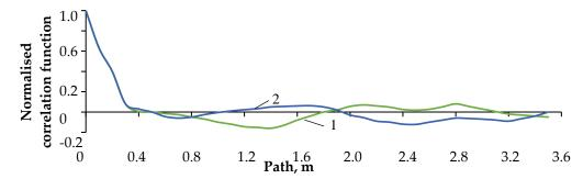
Fig. 4. Normalized correlation functions of fluctuations in the distance between the plants in a row of crops: 1 – autumn-sown sunflower; 2 – sunflower, grown using the conventional technology
